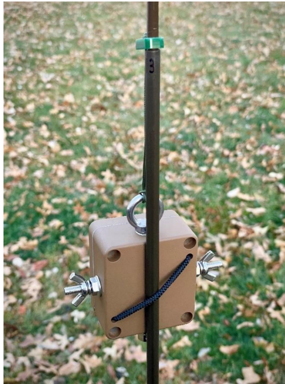
Figure 5: Use of the Arete COBRA's shock cord stabilizer with a portable fiberglass mast.
